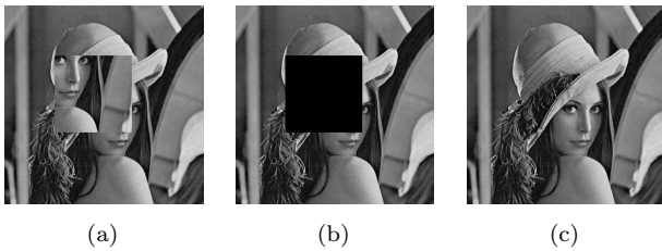
Figure 9. Image of Lena: (a) 15% tampered; (b) the detected tampered regions; (c) recovered image
